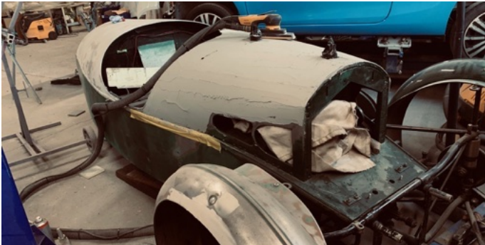
26th September 2025. Panel beating complete, filling and fitting now in progress.
