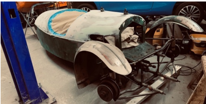
20th January 2026. Filling and flattening completed (if you can see any difference !) and more or less ready for the paint booth.
