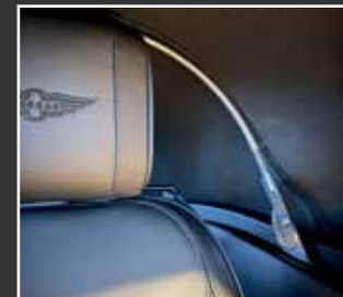
CLEVER SOFT TOP TENSIONER FOR THE MORGAN SUPERSPORT
